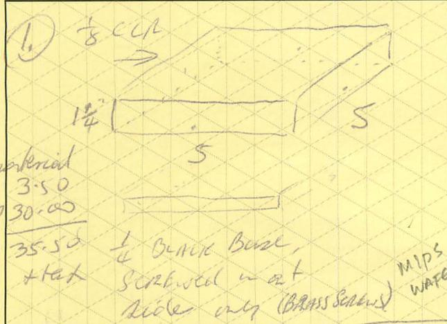
2. Make base (1/4 BLACK) for 5x7 UNFRAME, (BRASS) SCREENS on 4 sides, mount CIRCUIT BOARD to Base w/BRASS SCREWS.
